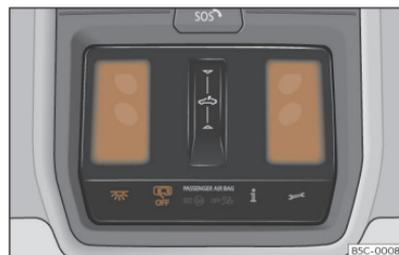
**Fig. 105** Detail of headliner: front interior lighting.
