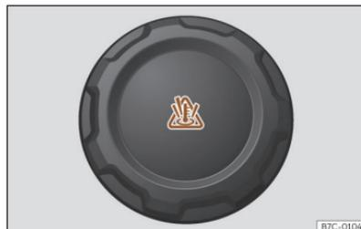
**Fig. 192** Front compartment: coolant expansion tank cap.
