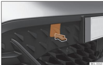
**Fig. 183** Front bumper on right: remove the lid.
