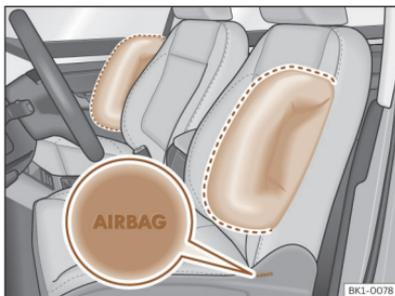
**Fig. 47** Driver's seat and passenger seat side airbags.
