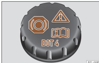
**Fig. 193** Front compartment: brake fluid reservoir cap.
