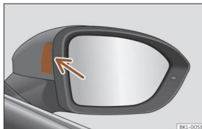
**Fig. 138** Control lamp of the lane departure warning.
