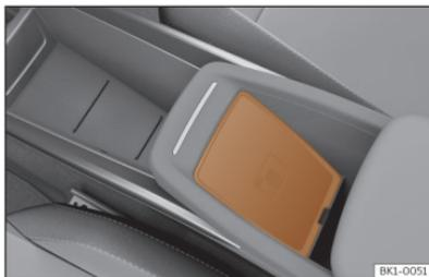
**Fig. 167** Centre console: slot for mobile phone connection.
