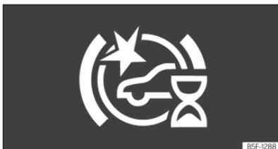
**Fig. 131** On the instrument cluster screen: indication of the system's initial self-calibration.
