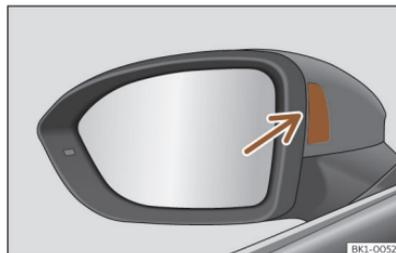
**Fig. 137** Control lamp of the lane departure warning.
