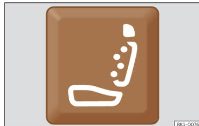
**Fig. 102** On the lateral underside of the driver and passenger seats: massage function button.
