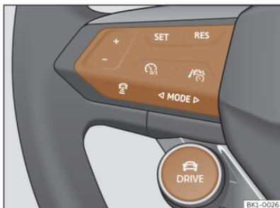
Fig. 92 Controls on the steering wheel.
