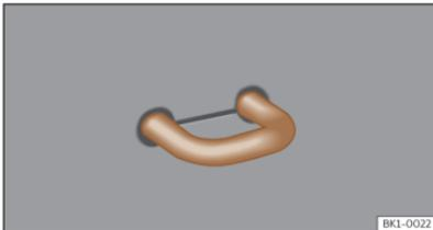
**Fig. 173** In the luggage compartment: fastening rings.
