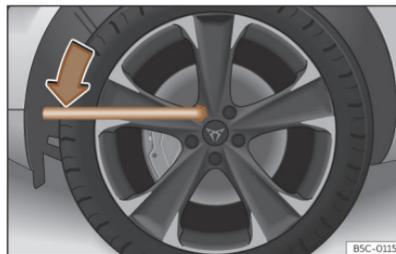
**Fig. 200** Tyre change: slacken the wheel bolts.
