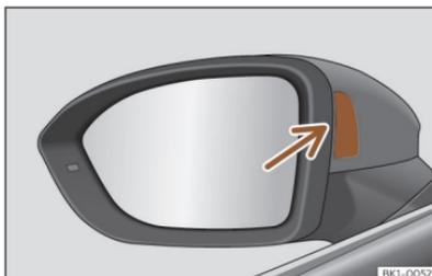
Fig. 156 On the mirror: warning lamp.
