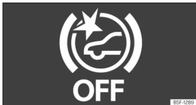
**Fig. 132** On the screen of the instrument panel Front Assist switched off message.
