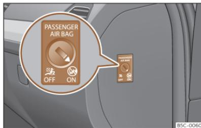
**Fig. 43** Switch for activating and deactivating the front passenger airbag.
