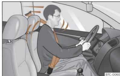
**Fig. 33** Drivers with properly worn seat belts will not be thrown forward in the event of sudden braking.
