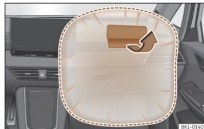
**Fig. 42** Front passenger airbag located in dash panel.
