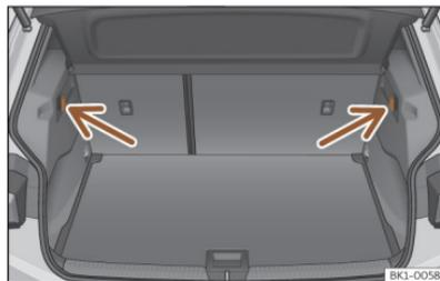
**Fig. 174** In the boot: retaining hooks.
