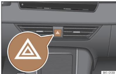
**Fig. 60** Dashboard: switch for hazard warning lights.
