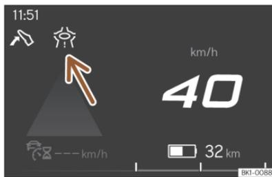
**Fig. 25** Eco-efficient driving assistance indication (schematic representation).
