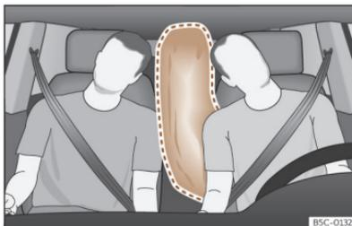
**Fig. 46** Fully inflated central airbag (deployment zone).
