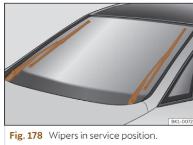
**Fig. 178** Wipers in service position.
