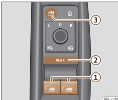
**Fig. 91** Detail of the driver door: controls for the windows.
