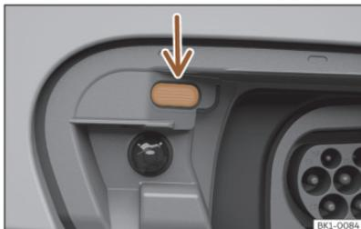
**Fig. 18** Charging process indicator LED
