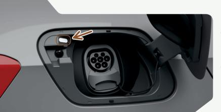
The connector remains locked during the charging process.
